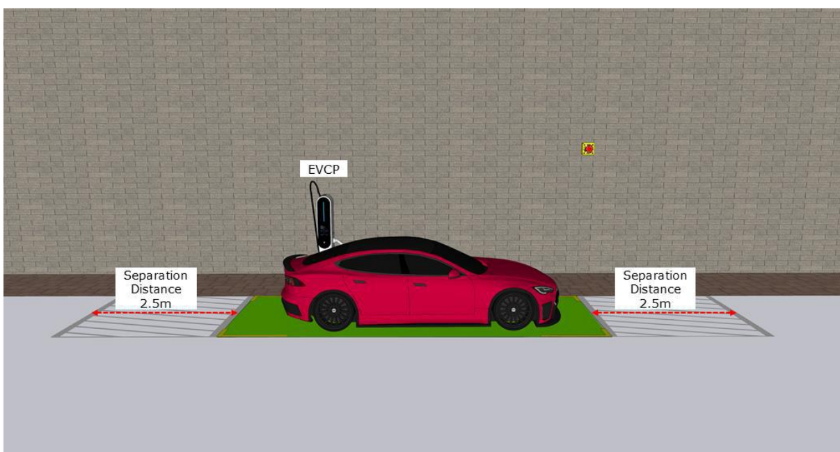
Figure 6: EVCB with DC Charger Located outdoors should be Separated with a Distance of 2.5 m from Non-EV Parking Bay
