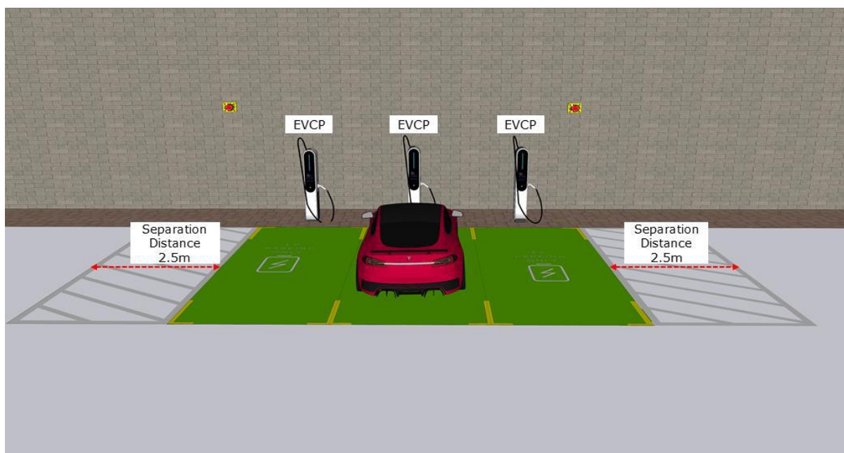
Figure 5: EVCB with AC Charger Located Outdoor in New Development should be Separated by a Distance of 2.5m from Non-EV Parking Bay
